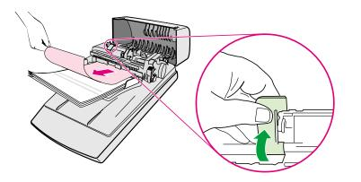
3 If the item cannot be easily removed, lift the two green tabs located behind the rollers and gently remove the green paper lead as shown.
